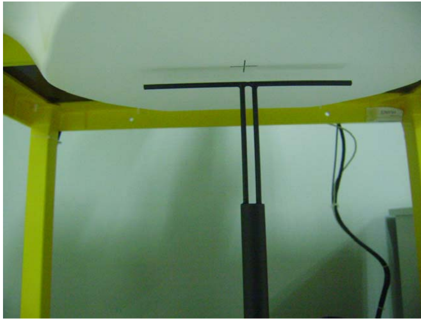
Setup Photo of Dipole Antenna
