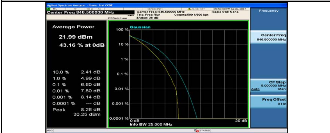
(Channel Bandwidth: 5 MHz)_HCH_QPSK_25RB#0
