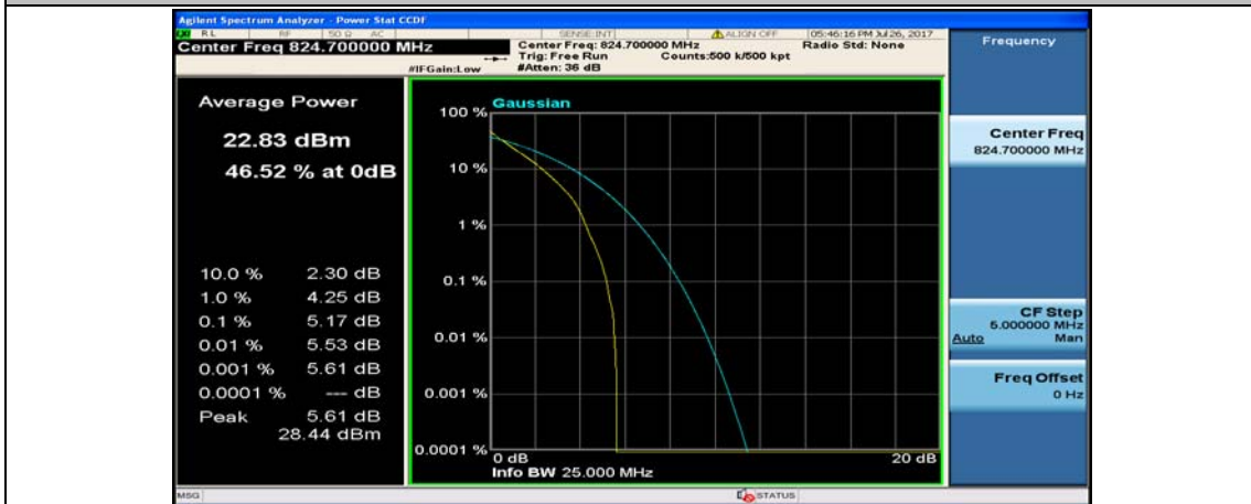
(Channel Bandwidth: 1.4 MHz)_LCH_QPSK_6RB#0
