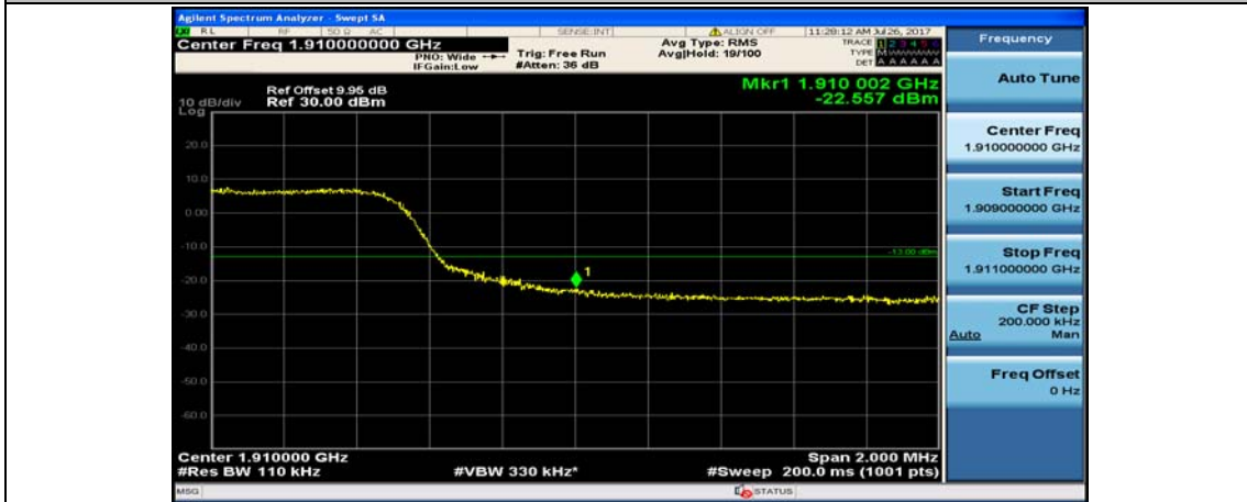
Channel Bandwidth: 10 MHz_HCH_16QAM_50RB#0
