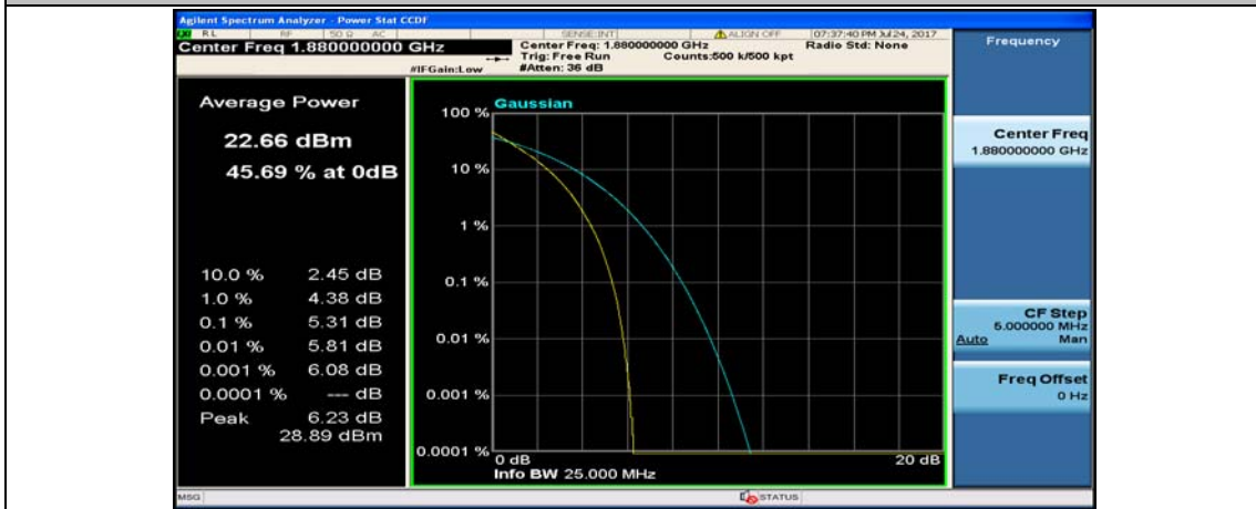
(Channel Bandwidth:20 MHz)_MCH_QPSK_100RB#0
