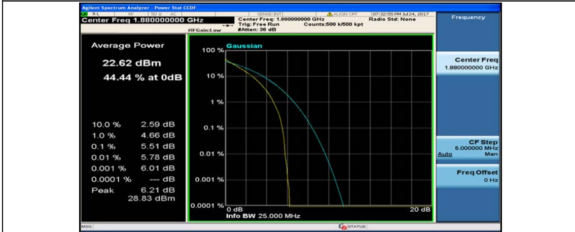
(Channel Bandwidth:15 MHz)_MCH_QPSK_75RB#0
