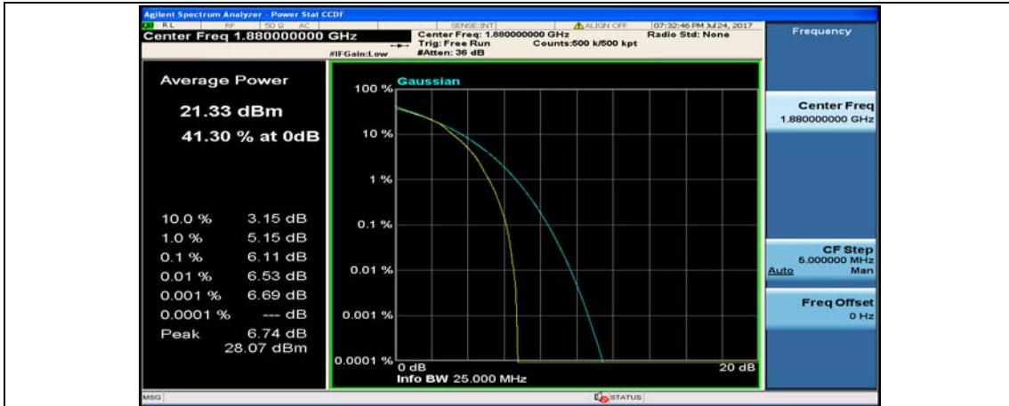
(Channel Bandwidth:15 MHz)_MCH_16QAM_75RB#0
