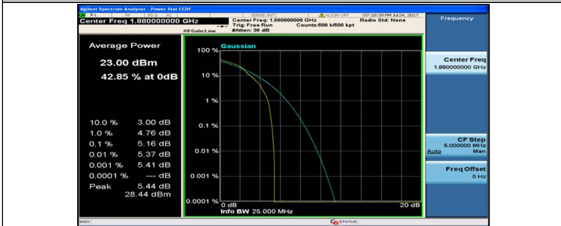
(Channel Bandwidth: 5 MHz)_MCH_16QAM_1RB#24
