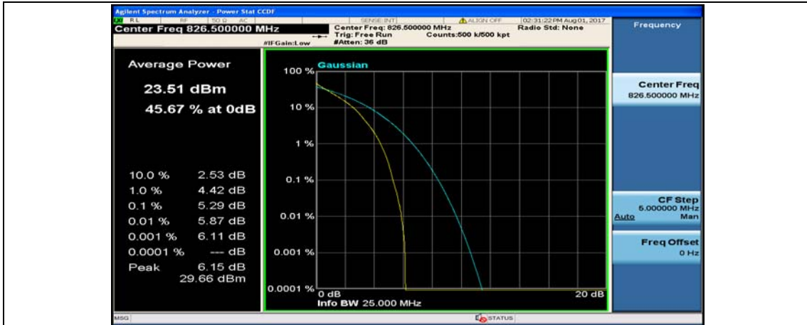
(Channel Bandwidth: 5 MHz)_LCH_QPSK_12RB#6
