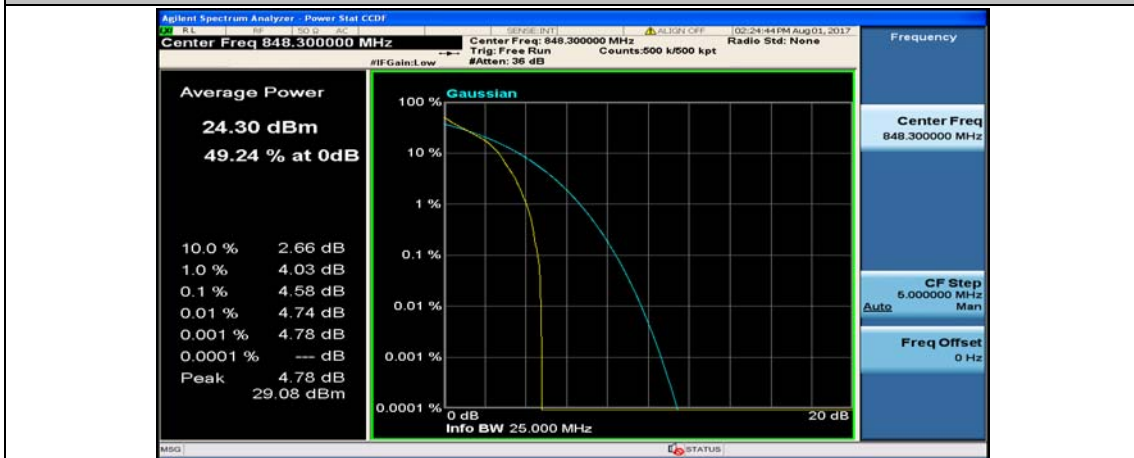
(Channel Bandwidth: 1.4 MHz)_HCH_QPSK_1RB#3
