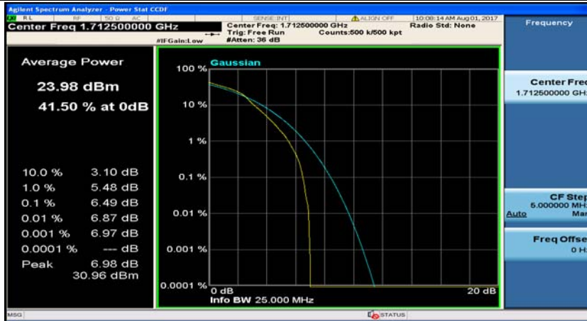
(Channel Bandwidth: 5 MHz)_LCH_16QAM_1RB#12
