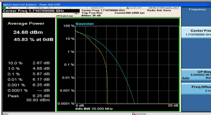
(Channel Bandwidth: 1.4 MHz)_LCH_QPSK_3RB#0
