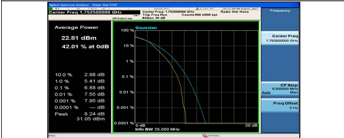
(Channel Bandwidth: 5 MHz)_HCH_16QAM_12RB#6
