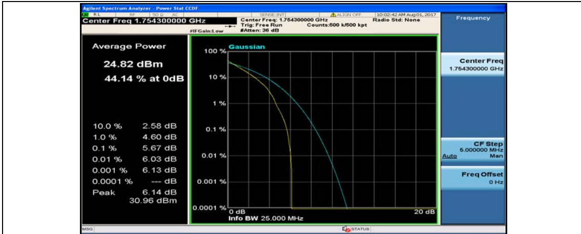
(Channel Bandwidth: 1.4 MHz)_HCH_QPSK_3RB#3
