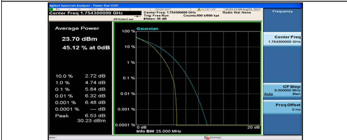
(Channel Bandwidth: 1.4 MHz)_HCH_QPSK_6RB#0
