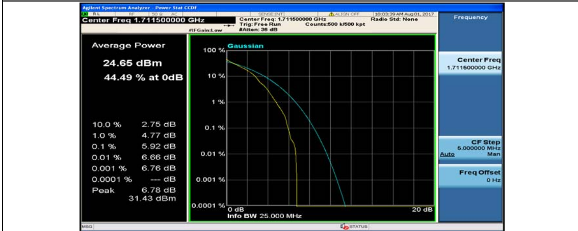
(Channel Bandwidth: 3 MHz)_LCH_QPSK_8RB#0
