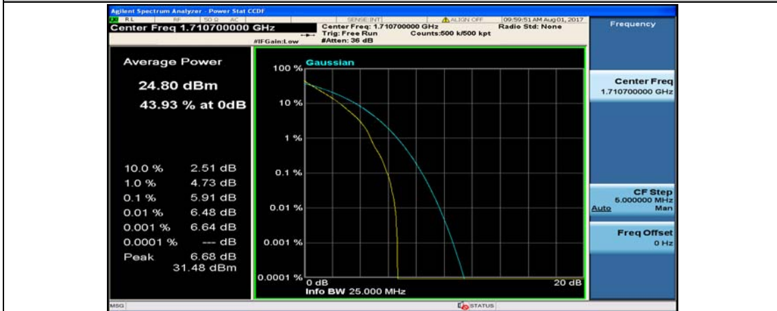
(Channel Bandwidth: 1.4 MHz)_LCH_QPSK_6RB#0
