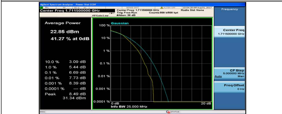
(Channel Bandwidth: 3 MHz)_LCH_16QAM_8RB#7
