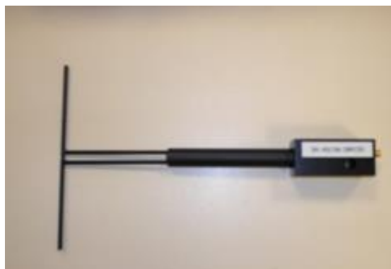
Figure 1 – Satimo COMOSAR Validation Dipole
