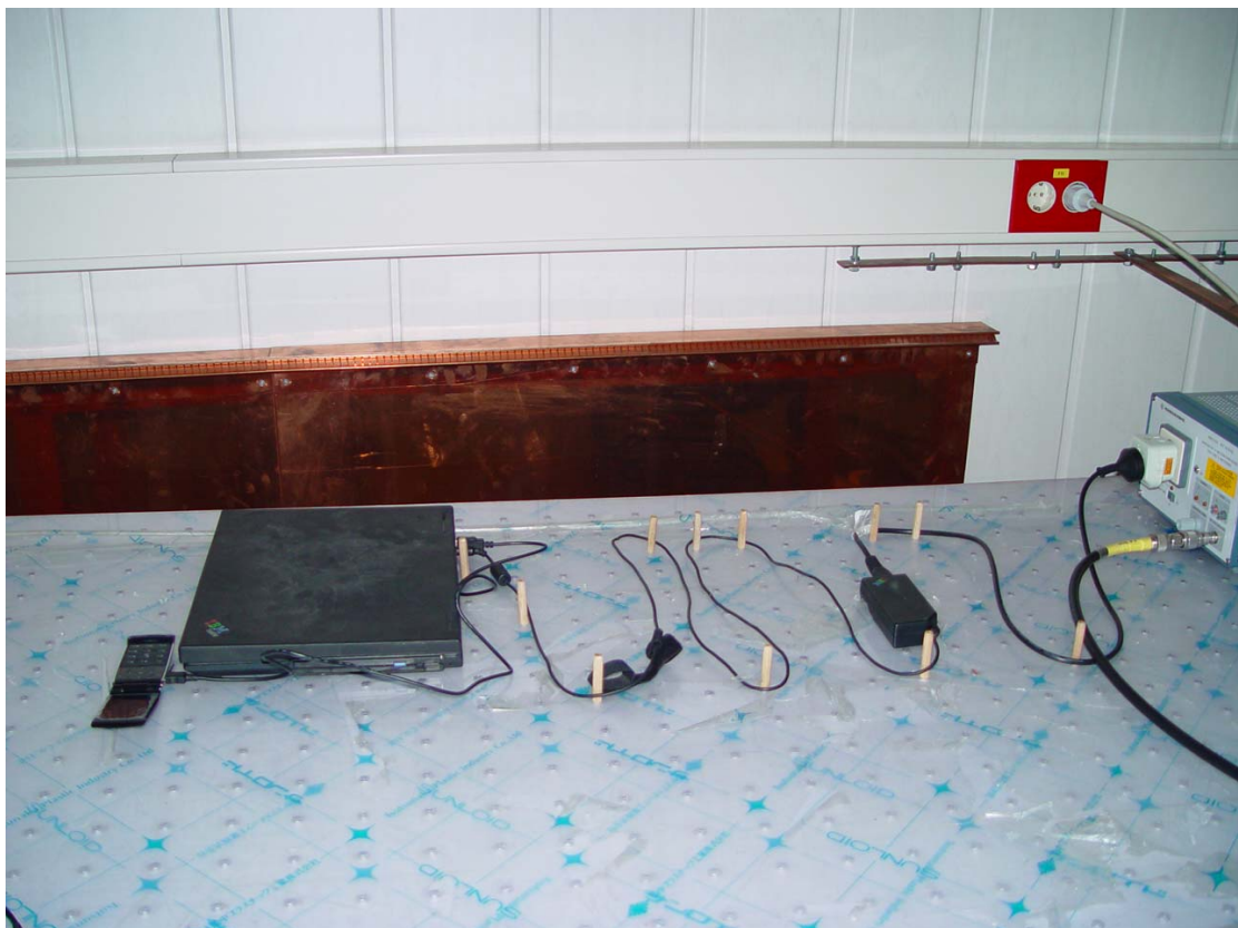
Pic 2 Conducted Emissions Test Setup
