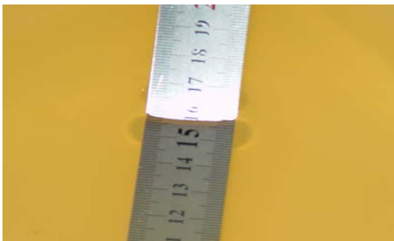
Liquid depth for SAR Measurement
