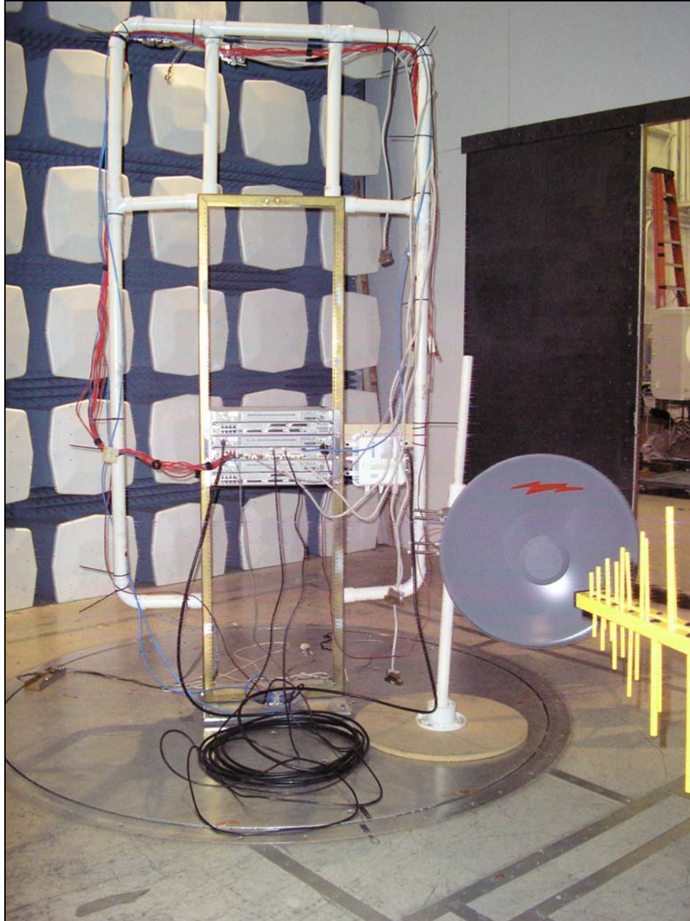
Photograph 1. Radiated Emission Limits Test Setup
