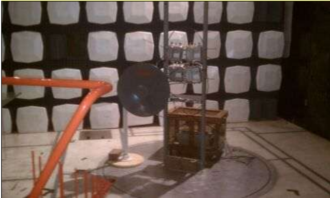
Photograph 1. Radiated Emissions, Test Setup, LF
