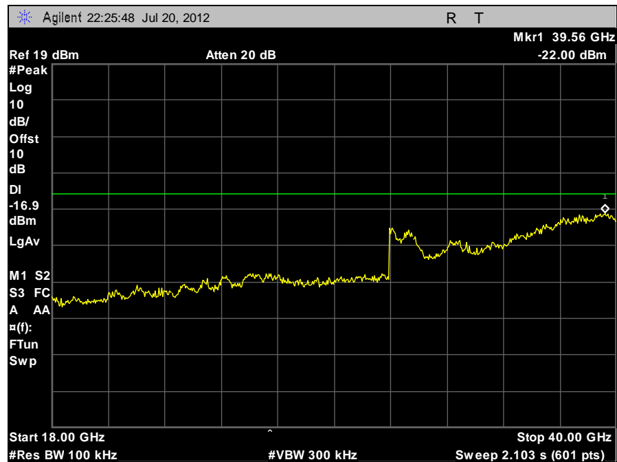
Plot 36. Conducted Spurious Emissions, 5818 MHz, 18 GHz – 40 GHz
