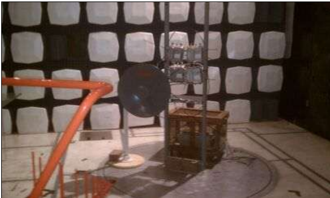
Photograph 3. Radiated Spurious Emissions, Test Setup, LF
