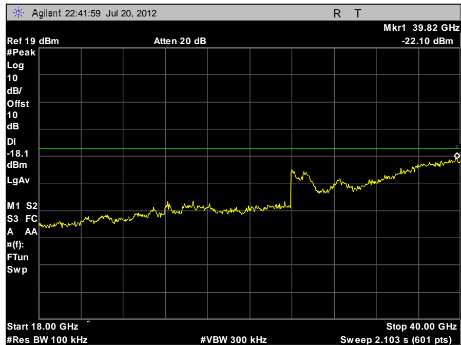
Plot 34. Conducted Spurious Emissions, 5757 MHz, 18 GHz – 40 GHz
