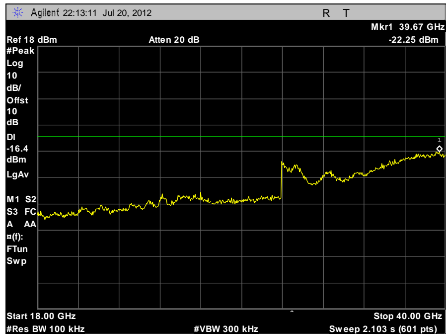
Plot 38. Conducted Spurious Emissions, 5834 MHz, 18 GHz – 40 GHz
