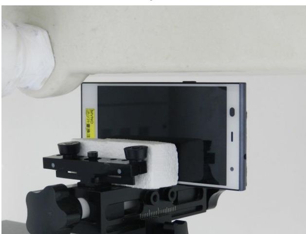
Left Side, Test Separation 10 mm
