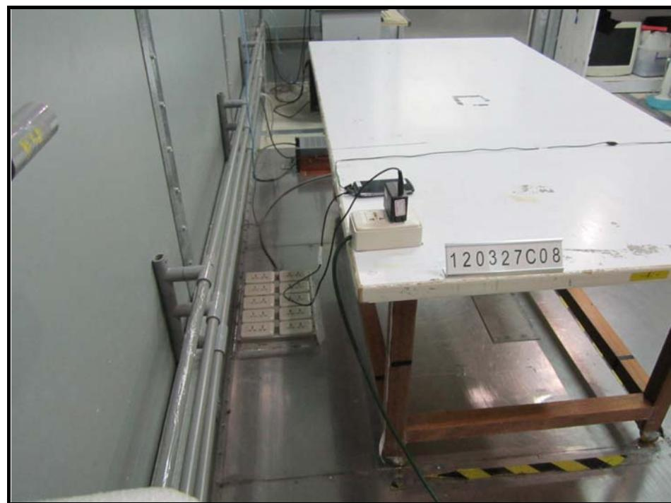
RADIATED EMISSION TEST (Y-Axis)
