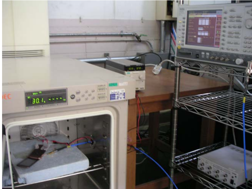
Temperature test (Frequency stability)
