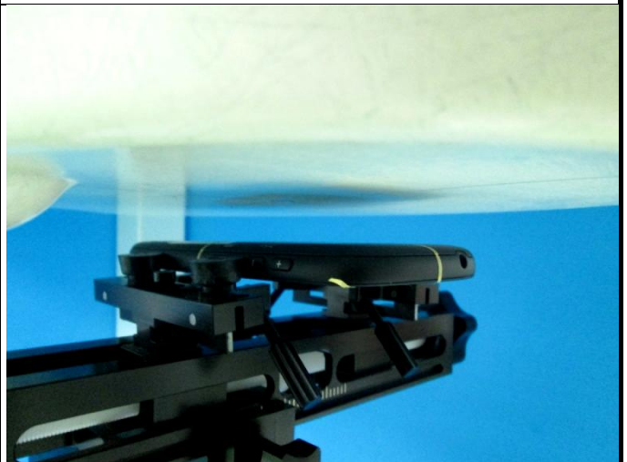
Rear Face of EUT with 1.5 cm Gap
