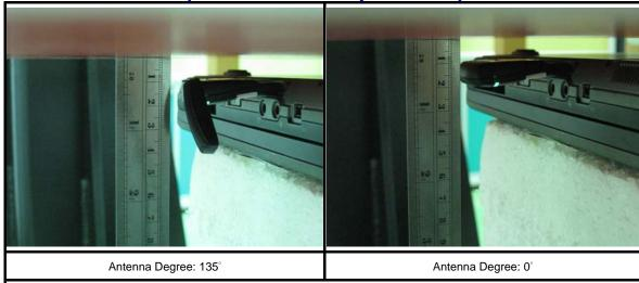
The bottom of the EUT face to the phantom with 10 mm-separation distance.
