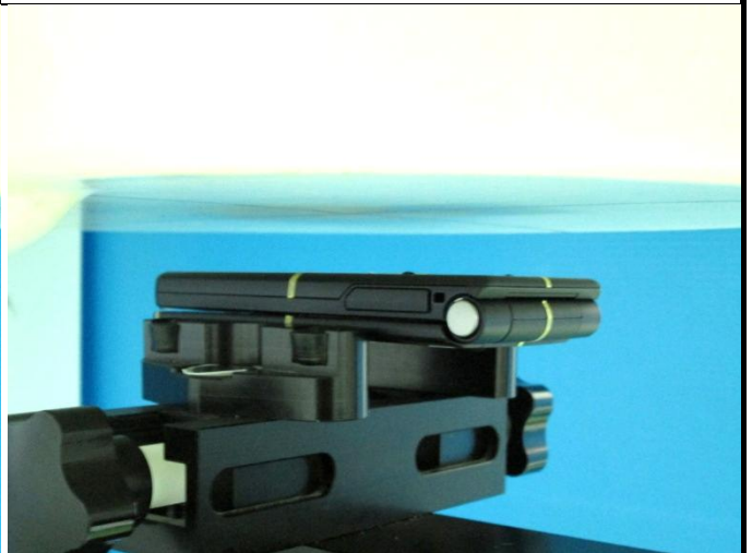
Rear Face of EUT with 1.5 cm Gap
