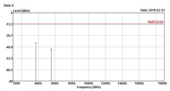
Site : 966 Chamber 5 Condition: PART22/24 VERTICAL Remak : PCS 1900 Link\_L-CH
