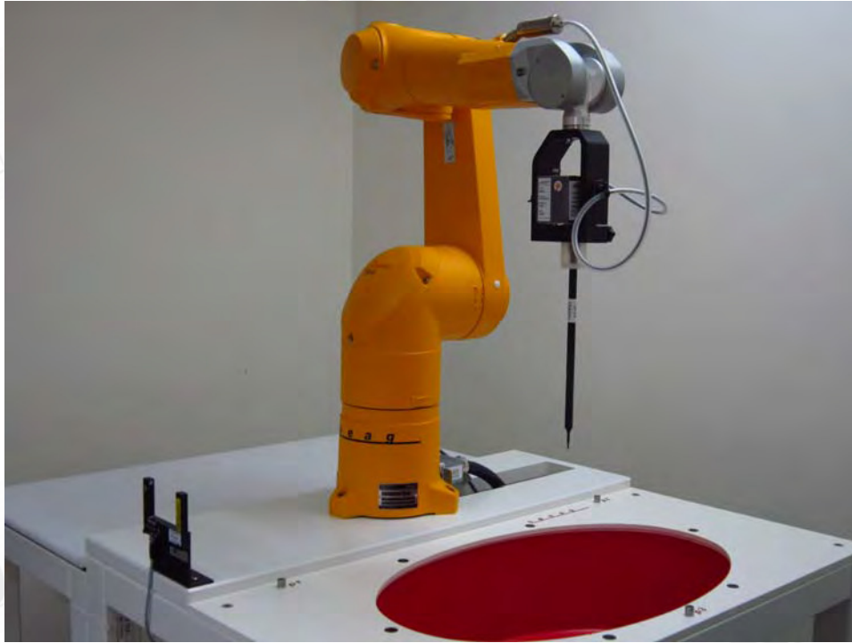
Fig.1 Photograph of the SAR measurement system
