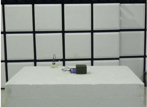
Radiated Emission Setup Photos (10~30MHz)
