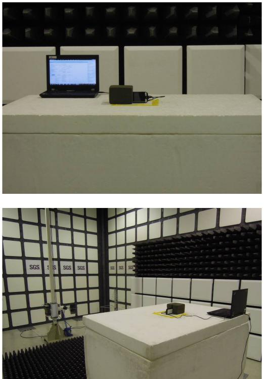
Radiated Emission Set up Photos (Above 1GHz)
