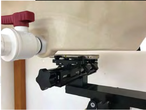
Fig.9 EUT Front side to flat phantom
