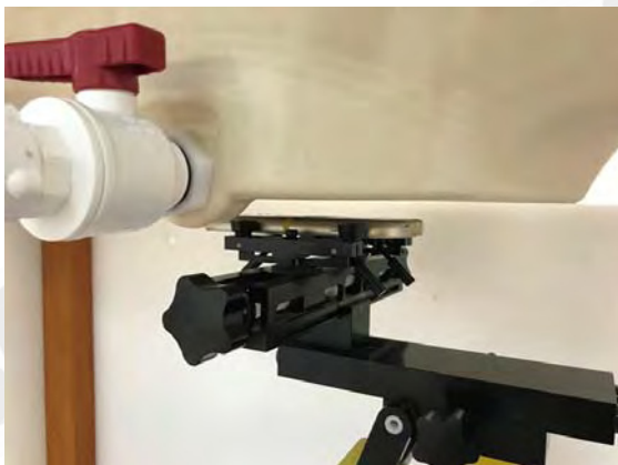
Fig.11 EUT Back side to flat phantom
