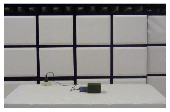
Radiated Emission Setup Photos (10~30MHz)
