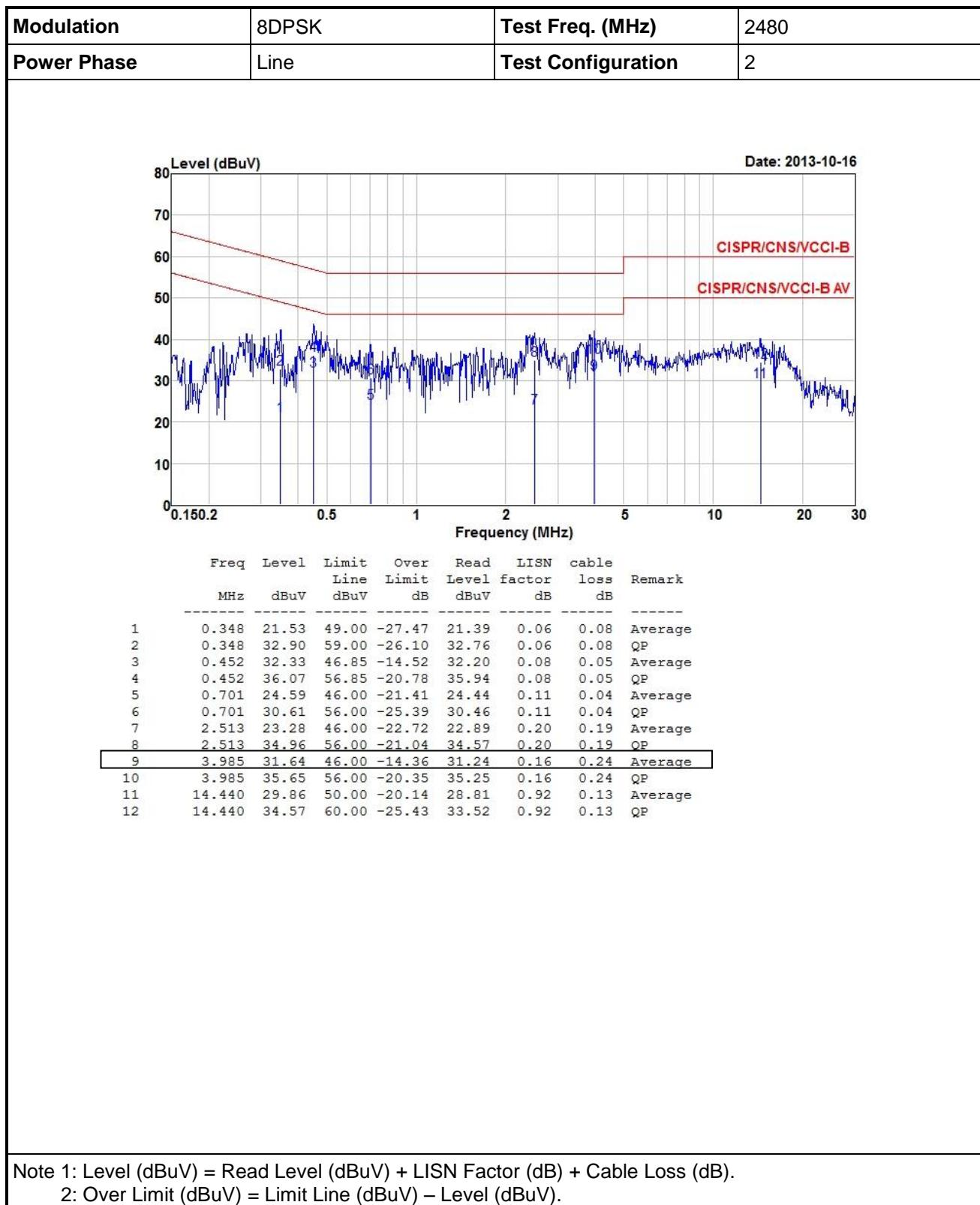
Note 1: Level (dBuV) = Read Level (dBuV) + LISN Factor (dB) + Cable Loss (dB).
