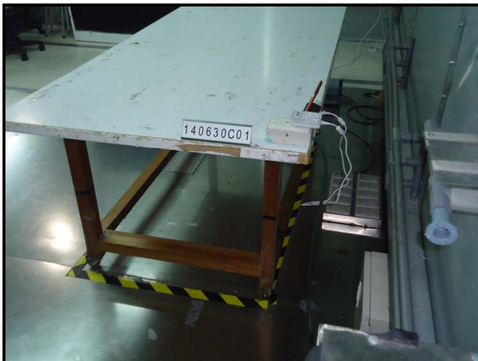
Radiated Emissions Test (Frequency range 30MHz~1GHz)
