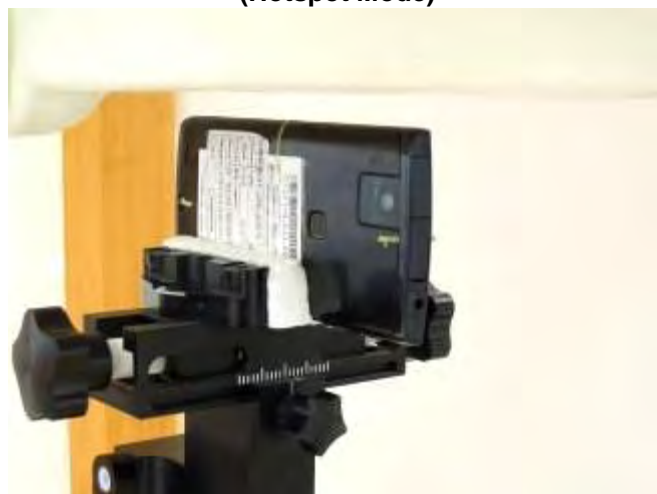
Right Side of EUT with 1 cm Gap (Hotspot Mode)
