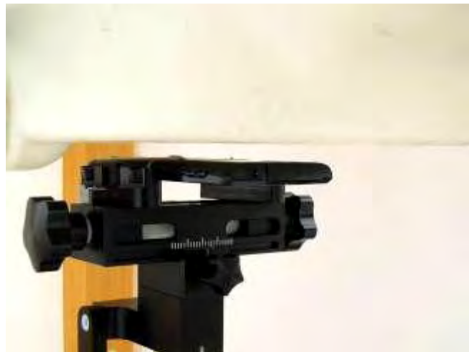
Rear Face of EUT with 1 cm Gap (Hotspot Mode)
