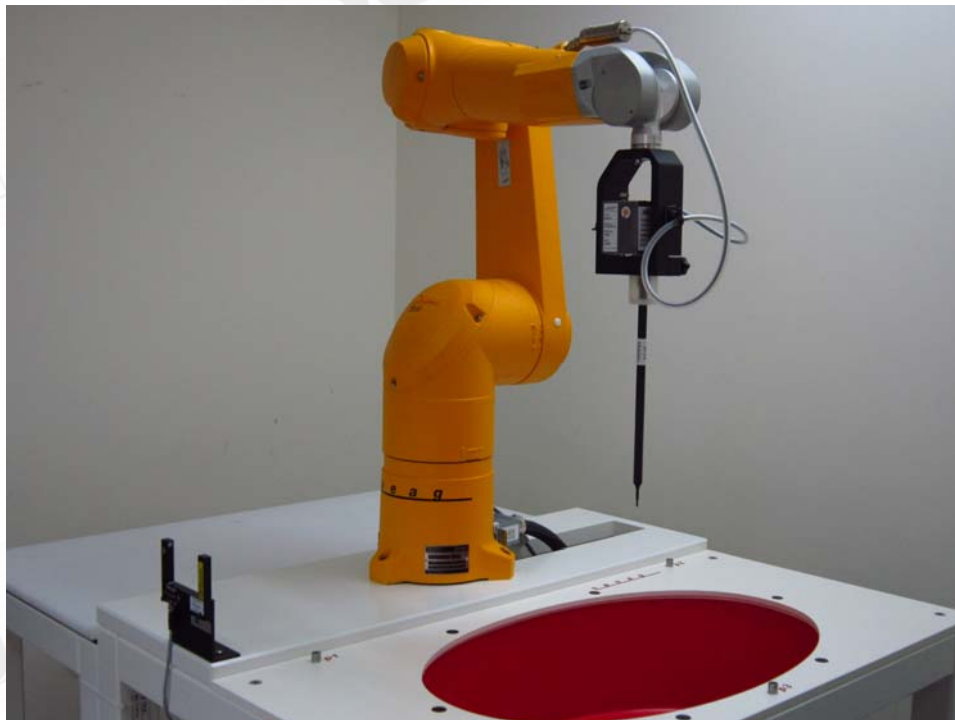
Fig.1 Photograph of the SAR measurement system
