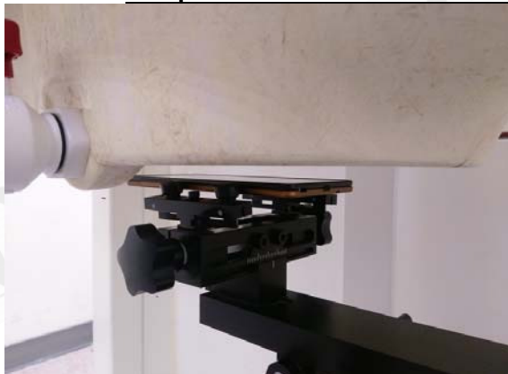
Fig.9 EUT Front side to flat phantom
