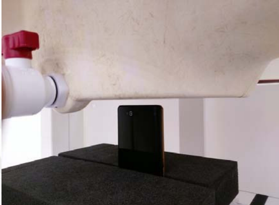
Fig.12 EUT Top side to flat phantom
