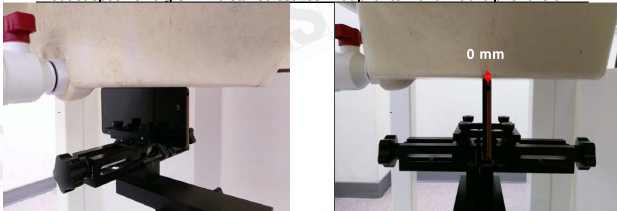
Fig.18 EUT Left side to flat phantom
