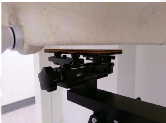
Fig.11 EUT Back side to flat phantom
