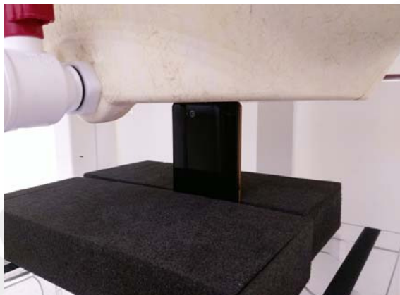
Fig.17 EUT Top side to flat phantom
