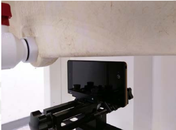
Fig.13 EUT Left side to flat phantom
