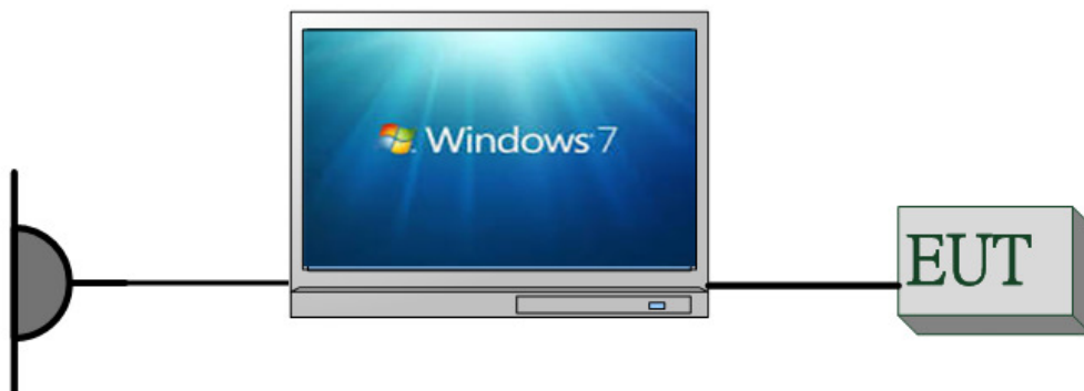
Fig. 2-1 Radiated Emission & Conducted (Antenna Port) Configuration
