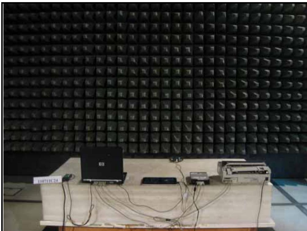
RADIATED EMISSION TEST (Y-Axis)
