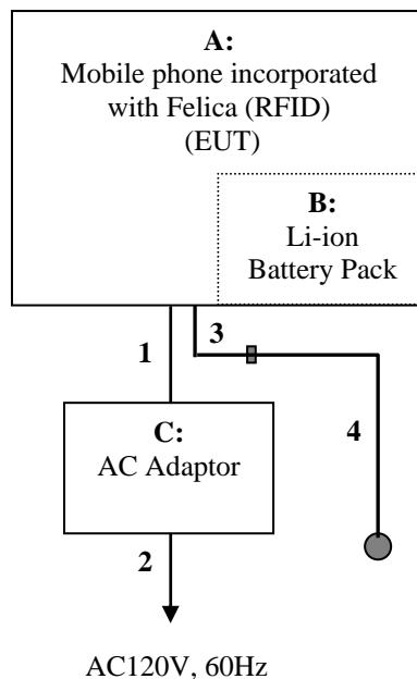
Note: EUT has one connector which is connected either AC adapter (No.1 and No.2 above) or Earphone (No. 3 and No.4 above). On each tests, the result of the worse condition is reported as worst case in this report.
