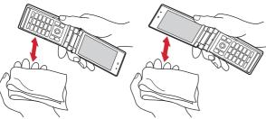
4 Remove the back cover and wipe off any drops of water around the inner lid and the rear side of the back cover. After wiping off the water, install and lock the back cover.
