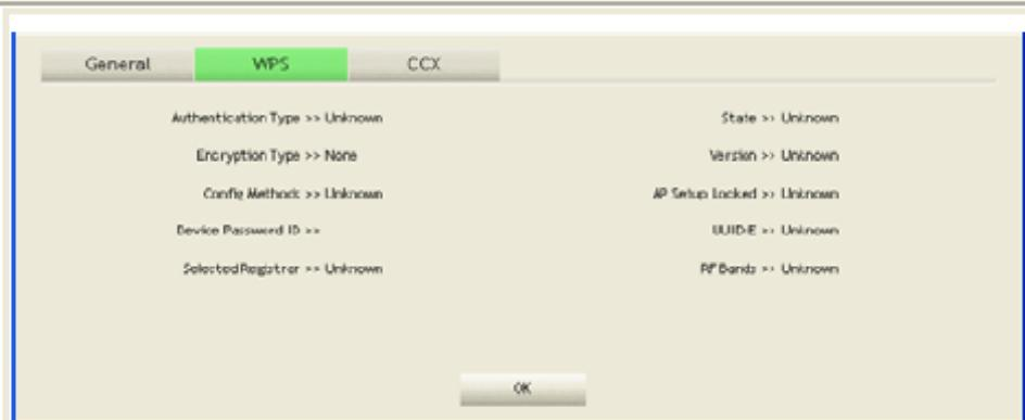
WPS information contains Authentication Type, Encryption Type, Config Methods, Device Password ID, Selected Registrar, State, Version, AP Setup Locked, UUID-E and RF Bands.
