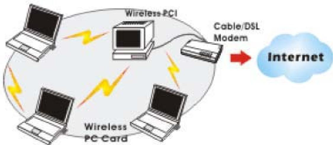
The Access Point Network The network installation allows you to share files, printers, and Internet access much more conveniently. With Wireless LAN Cards, you can connect wireless LAN to a wired global network via an Access Point.
