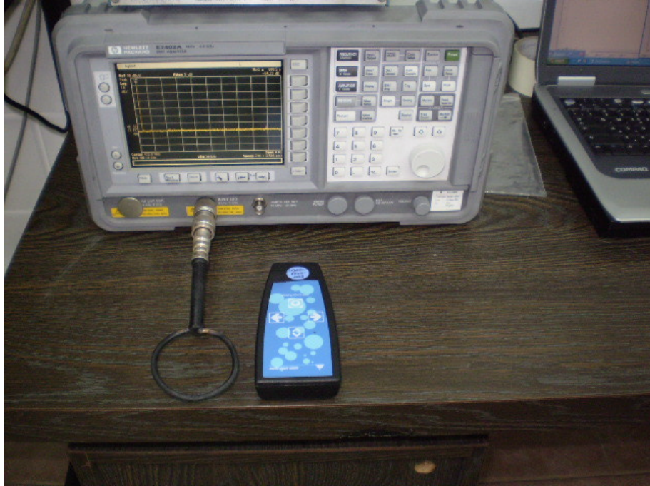
Photograph No.1 Occupied bandwidth measurement setup for RC0100200 controller
