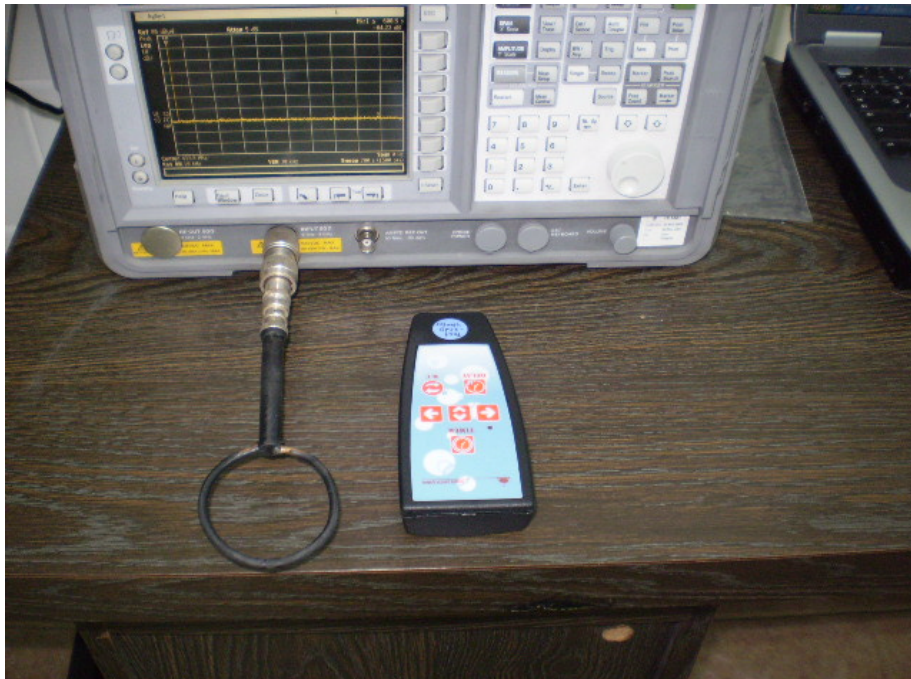
Photograph No.2 Occupied bandwidth measurement setup for RC0100100 controller
