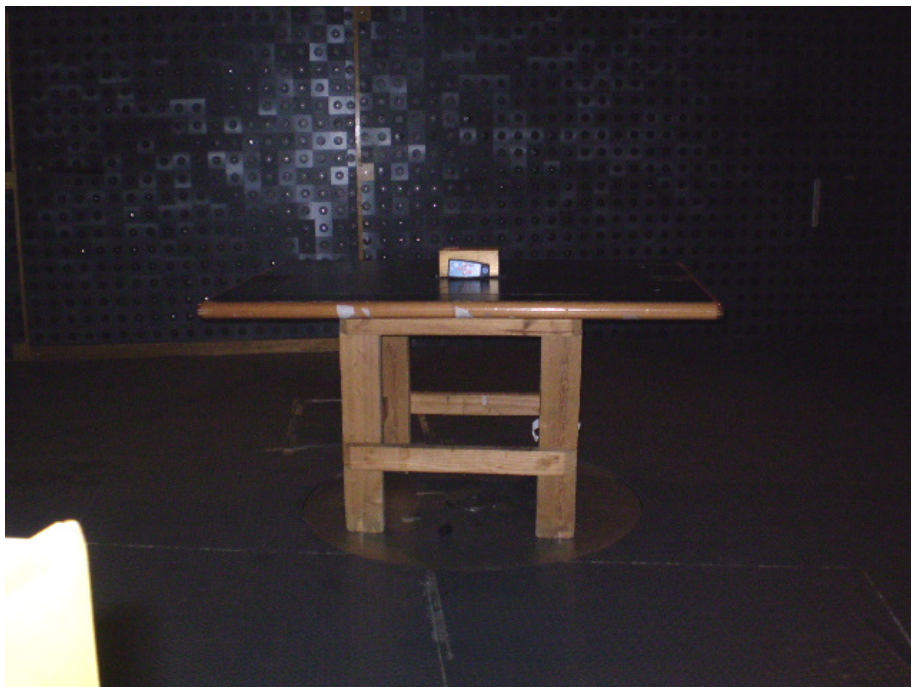
Photograph No.9 Spurious radiated emissions measurement setup in the anechoic chamber with double ridged guide antenna
