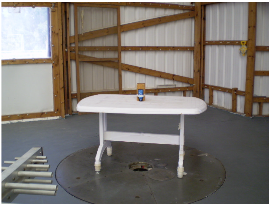
Photograph No.11 Spurious emission field strength measurement setup at the OATS with biconilog antenna, EUT in X-axis position
