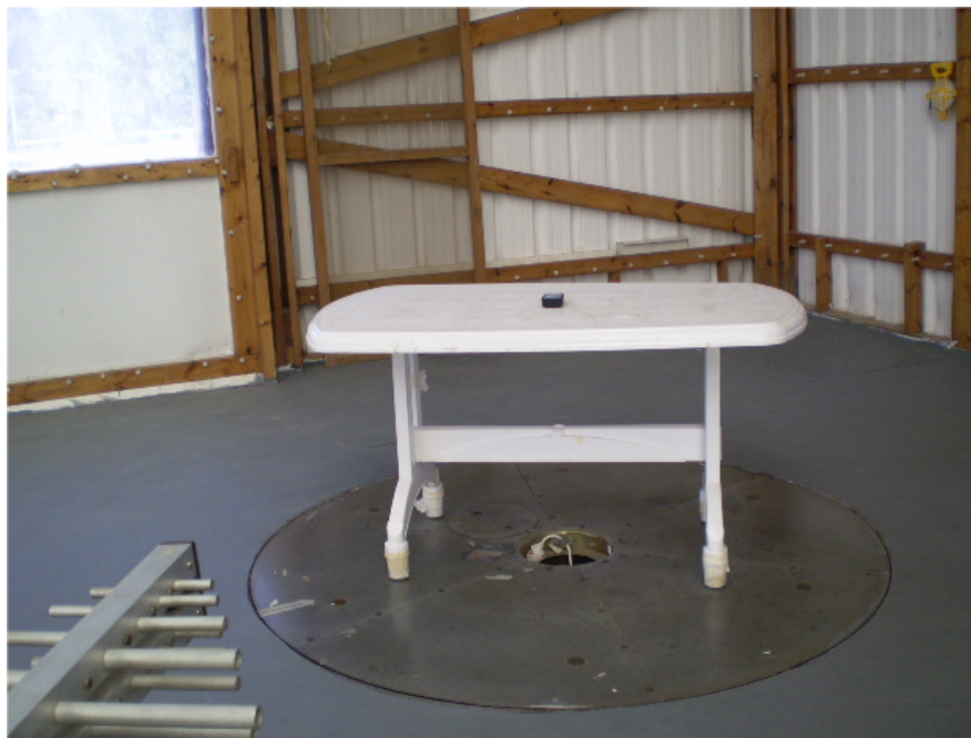
Photograph No.13 Radiated emission field strength measurement setup at the OATS with biconilog antenna, EUT in Z-axis position
