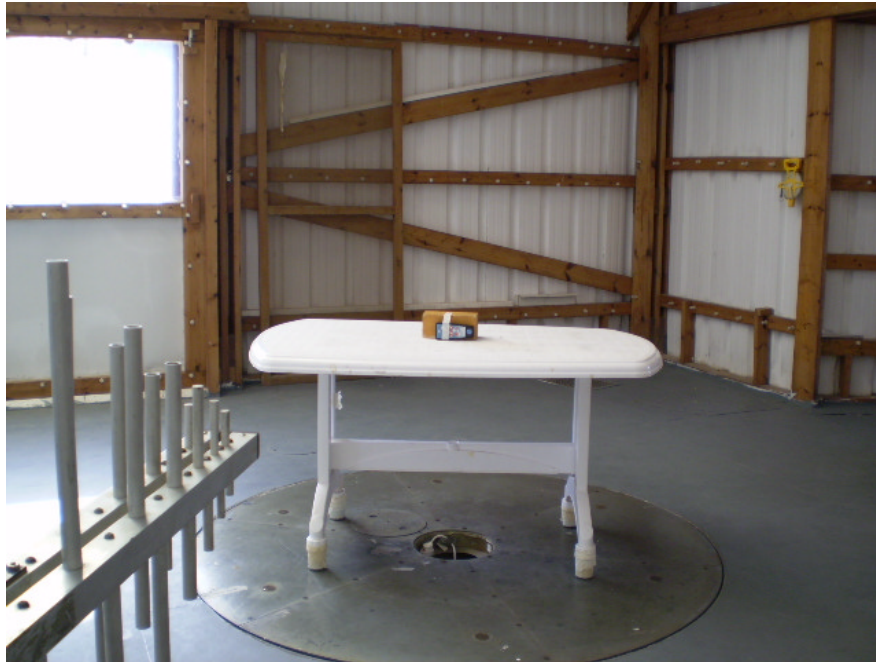
Photograph No.12 Radiated emission field strength measurement setup at the OATS with biconilog antenna, EUT in Y-axis position
