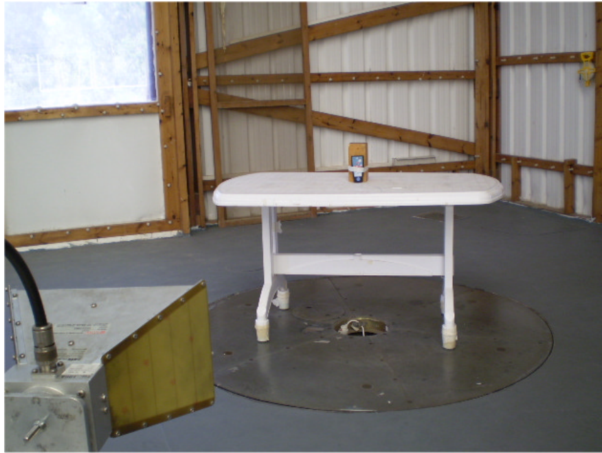
Photograph No.14 Spurious emission field strength measurement setup at the OATS with double ridged guide antenna, EUT in X-axis position
