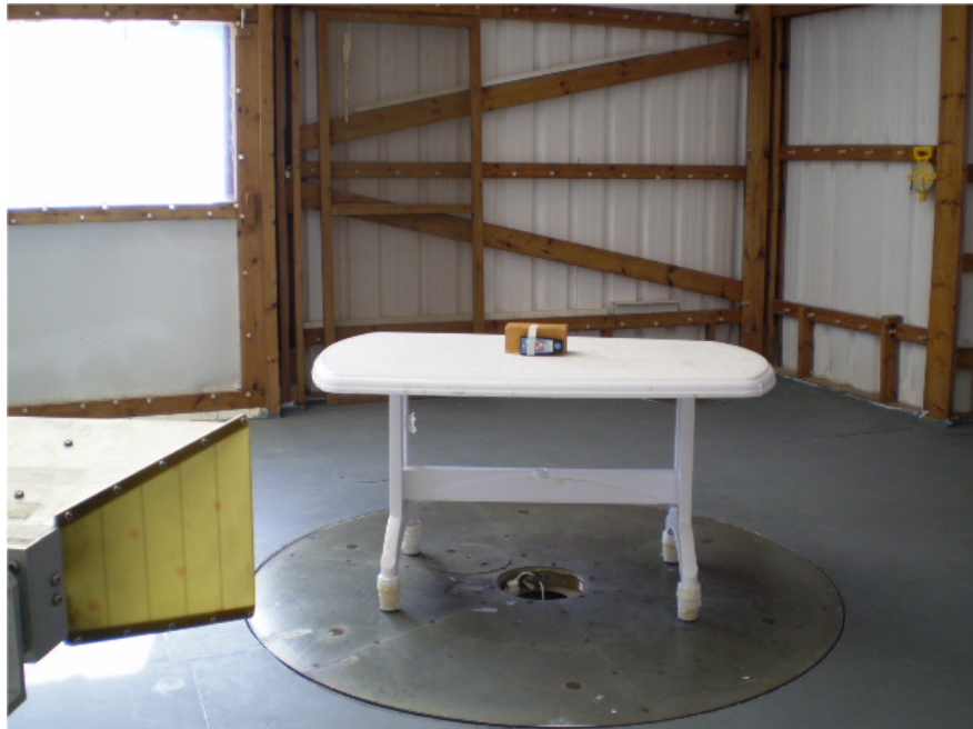
Photograph No.15 Spurious emission field strength measurement setup at the OATS with double ridged guide antenna, EUT in Y-axis position
