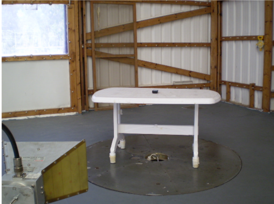
Photograph No.16 Spurious emission field strength measurement setup at the OATS with double ridged guide antenna, EUT in Z-axis position
