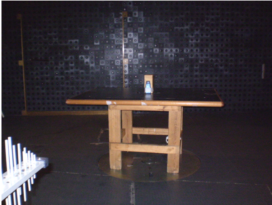
Photograph No.5 Radiated emissions measurement setup in the anechoic chamber in 30 MHz to 1000 MHz band
