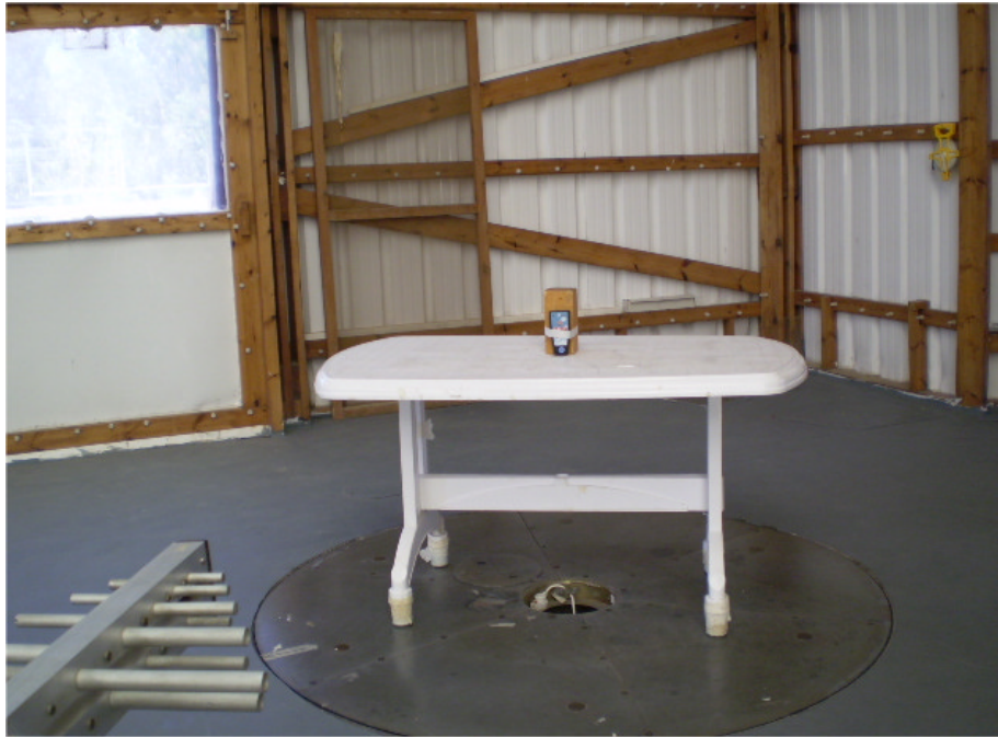
Photograph No.10 Radiated emission field strength measurement setup at the OATS with biconilog antenna, EUT in X-axis position
