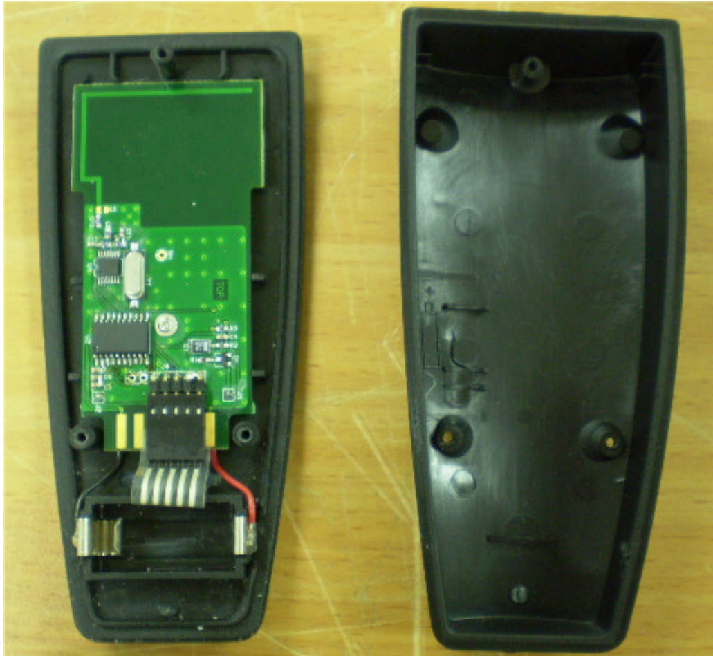
Photograph No.7 RC0100200 remote controller (4 buttons) Internal view
