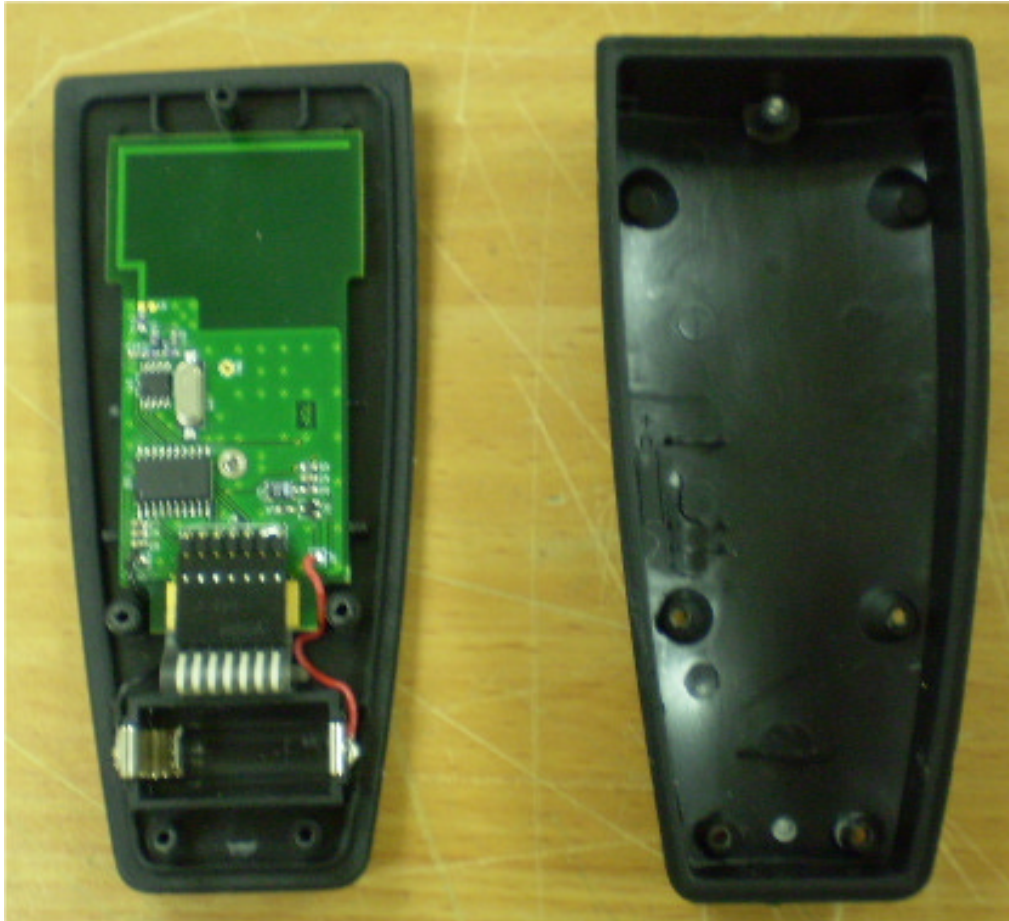
Photograph No.1 RC0100100 remote controller (6 buttons) Internal view with rear cover removed
