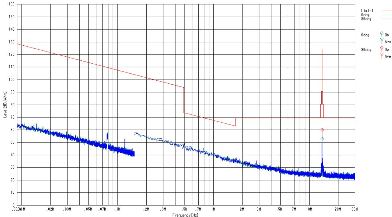
Note: 13.56 MHz is a Tx carrier. This is not spurious emission from EUT.
