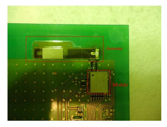
This module and antenna are concrete design, and approved according to KDB996369. The connection to the antenna is made through a host's printed board micro-strip trace layout to an trace antenna on a printed circuit board.
