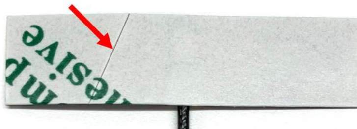
1. Find cut line on flex back side
