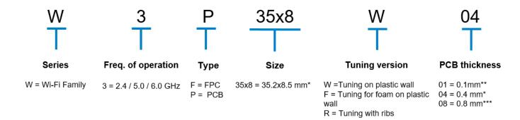
\*Typical thickness for PCB
