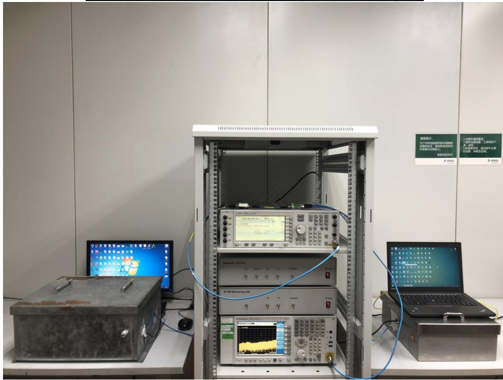
DFS Set-up Photo: Slave and Spectrum Analyzer
