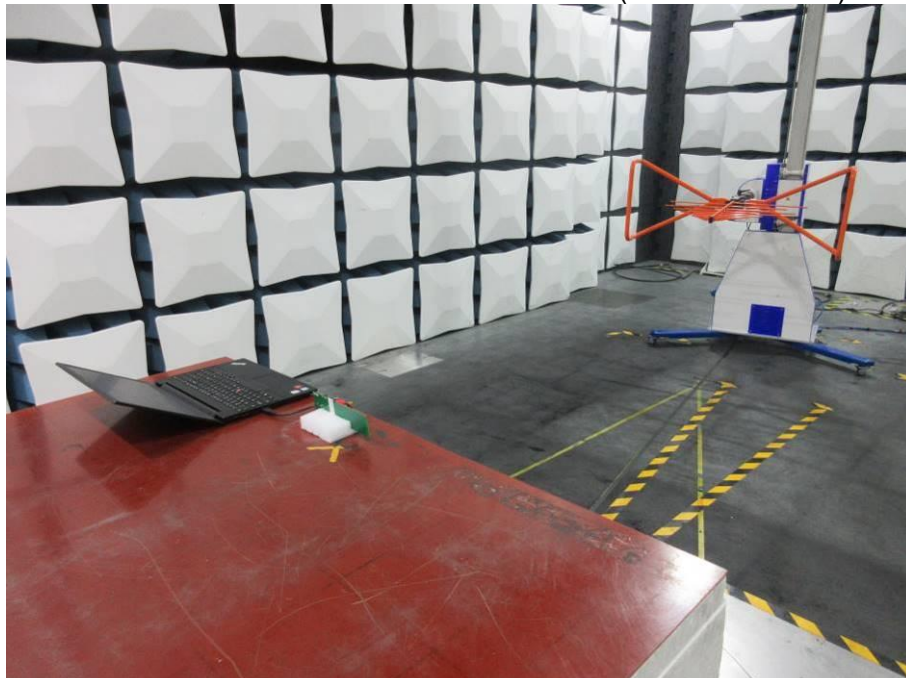
RADIATED RF MEASUREMENT SETUP (30MHz ~ 1 GHz)
