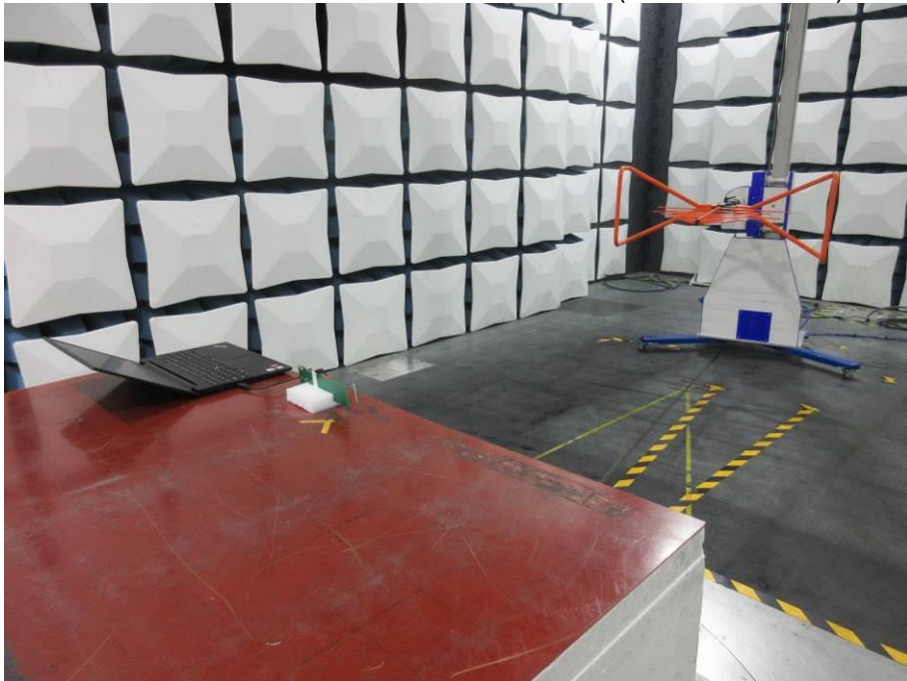
RADIATED RF MEASUREMENT SETUP (30MHz ~ 1 GHz)
