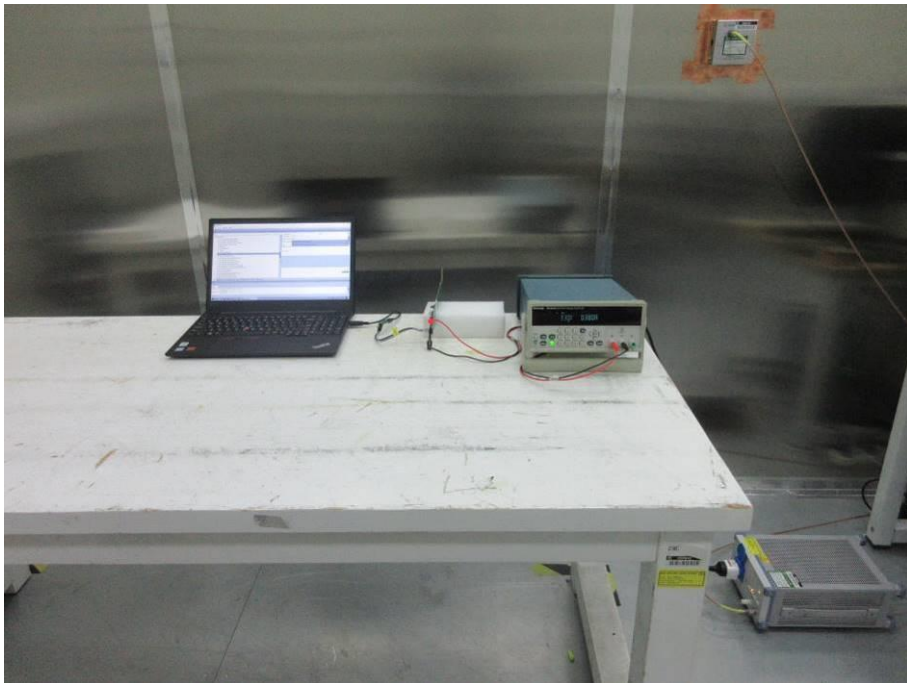
POWERLINE CONDUCTED EMISSIONS MEASUREMENT SETUP
