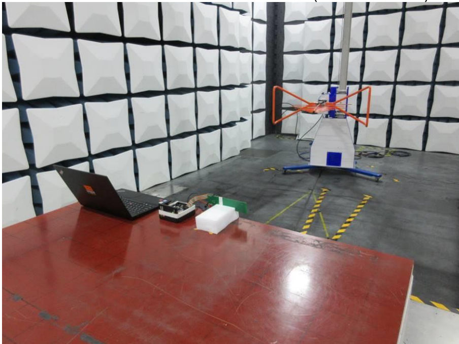
RADIATED RF MEASUREMENT SETUP (30MHz ~ 1 GHz)
