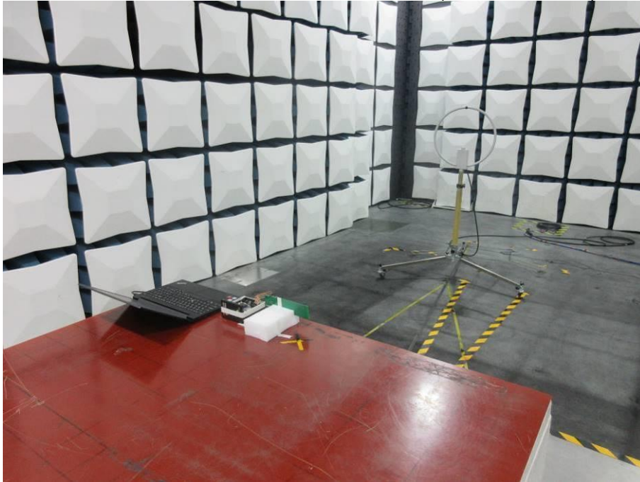
RADIATED RF MEASUREMENT SETUP (9KHz ~ 30 MHz)
