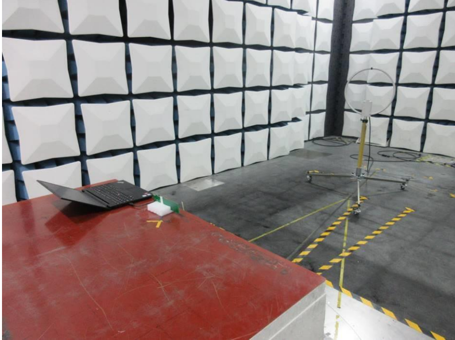
RADIATED RF MEASUREMENT SETUP (9KHz ~ 30 MHz)
