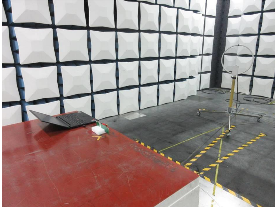
RADIATED RF MEASUREMENT SETUP (9KHz ~ 30 MHz)
