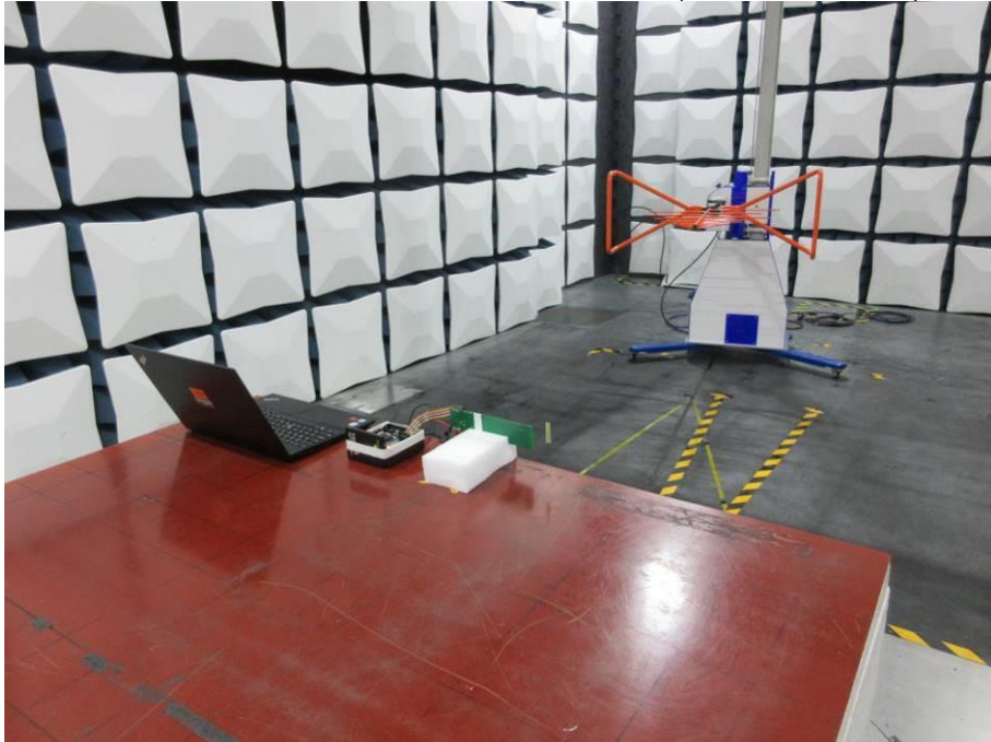
RADIATED RF MEASUREMENT SETUP (30MHz ~ 1 GHz)
