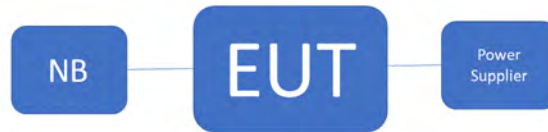
Fig. 2-3 Conducted (AC powerline) Emission Configuration
