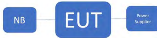
Fig. 2-2 Conducted (Antenna Port) Configuration Emission
