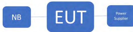
Fig. 2-3 Conducted (AC powerline) Emission Configuration
