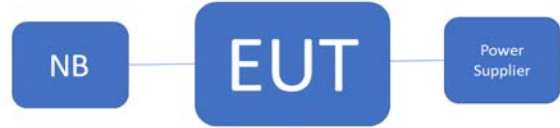
Fig. 2-2 Conducted (Antenna Port) Configuration
