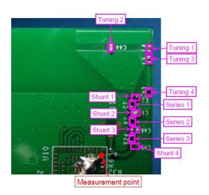
Different antenna length and shapes effect radiated emission and each design should be considered a different type: 2.4G WIFI:
