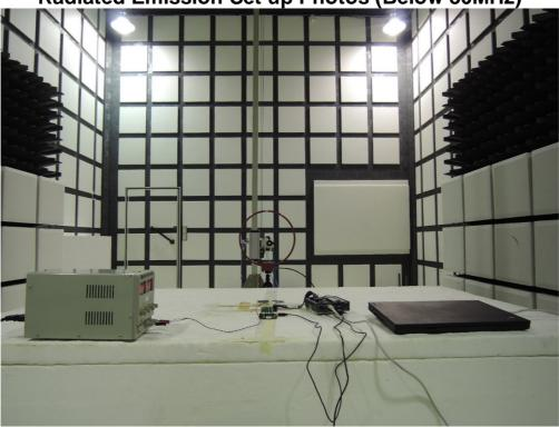
Radiated Emission Set up Photos (Below 1GHz)
