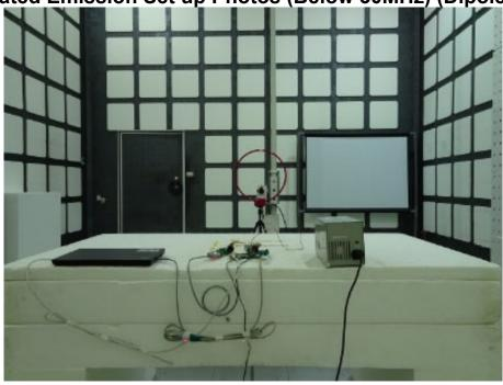
Radiated Emission Set up Photos (Below 1GHz) (Dipole Ant)
