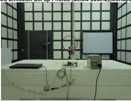
Radiated Emission Set up Photos (Below 1GHz) (Monopole Ant)
