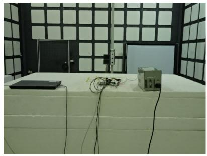
Radiated Emission Set up Photos (Below 1GHz) (Monopole Ant)
