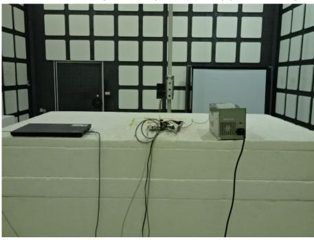
Radiated Emission Set up Photos(Front View) (SANT-Monopole Ant)
