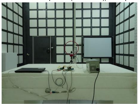
Radiated Emission Set up Photos (Below 1GHz) (SANT-Dipole Ant)
