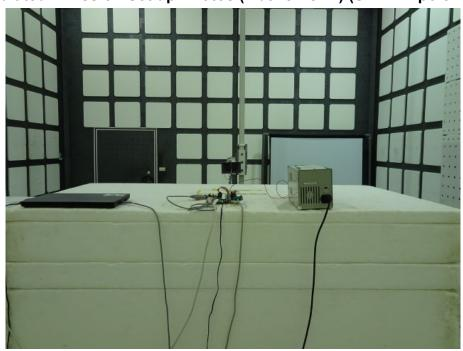
Radiated Emission Set up Photos(Front View) (SANT-Dipole Ant)
