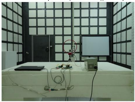
Radiated Emission Set up Photos (Below 1GHz) (DANT-Dipole Ant)
