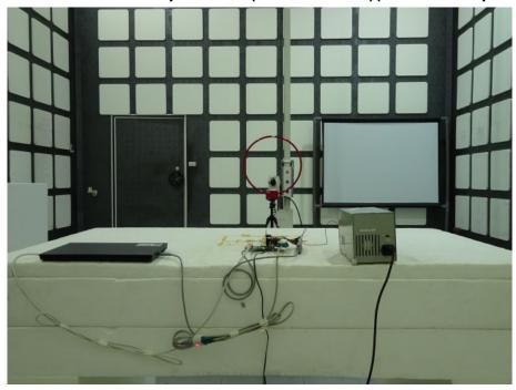
Radiated Emission Set up Photos (Below 1GHz) (SANT-Monopole Ant)
