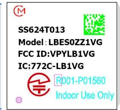
The labeling information is laser marked on the surface of shielding case of the module.
