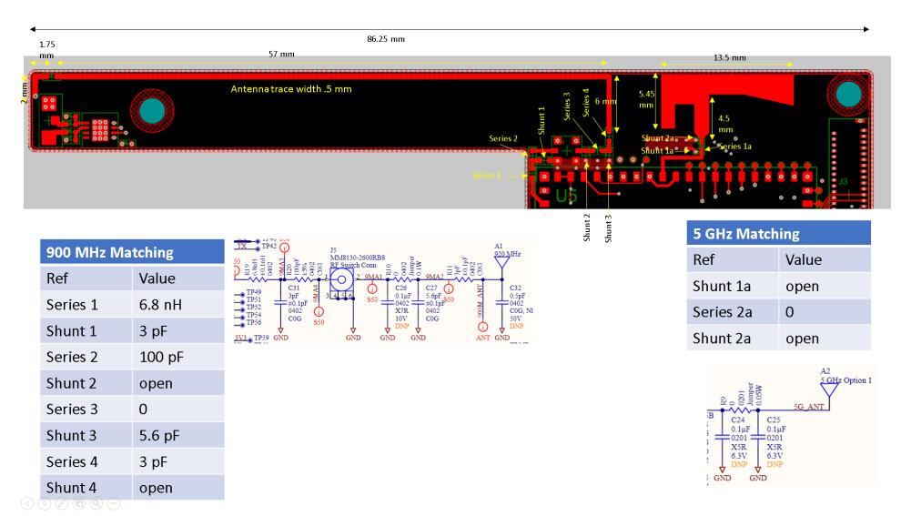
RF path of Monopole PCB antenna for 5GHz WLAN and sub-G
