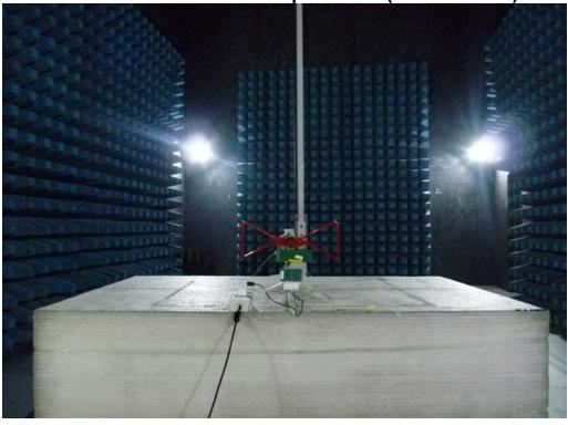
Radiated Emission Set up Photos (Above 1GHz)
